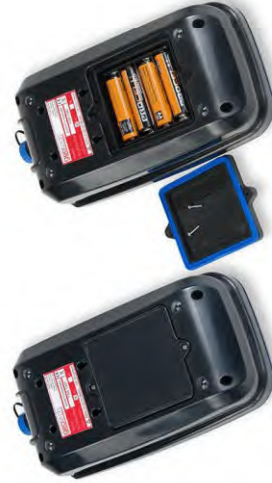
Figure 2-1: Replacing the batteries
