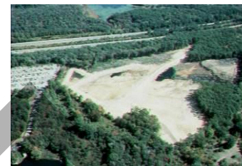
Hydraulic dredging containment area for Nutting Lake in Billerica: empty (above) and full (below) (provided by J. Walsh of BEC)
