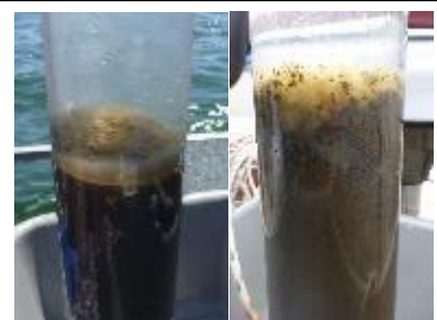
Floc layer visible on top of core samples 3 hours after treatment; layer will migrate into sediment within 2 months
