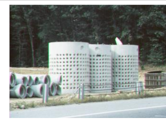
Leaching catch basin vaults
