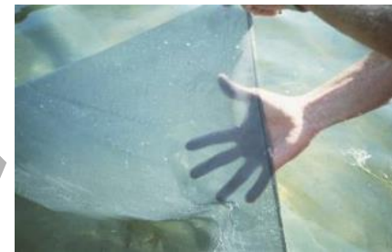
Porous weave benthic barrier (Aquascreen)
