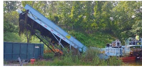
Mechanical harvester offloading to conveyor with transfer to rollaway hopper
