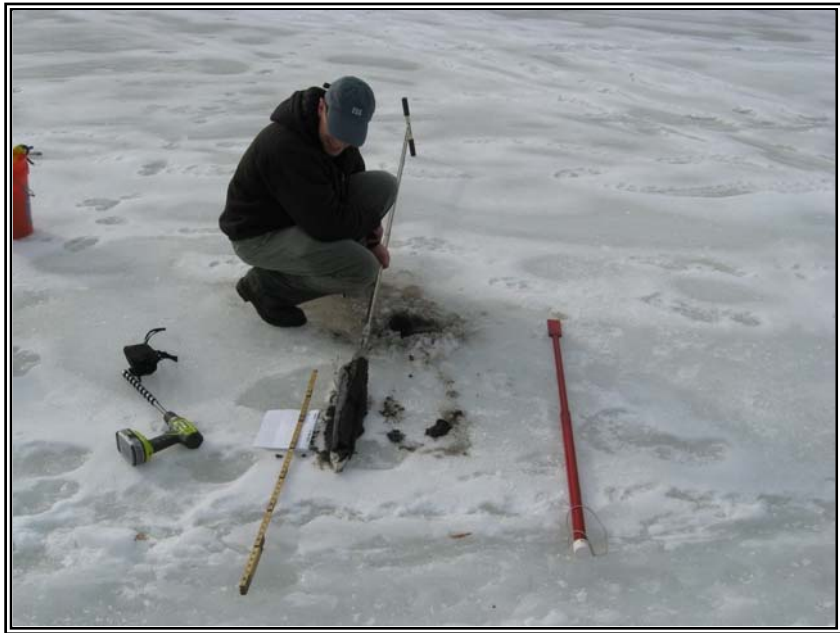
Photograph No. 4: Pulling core above ice
