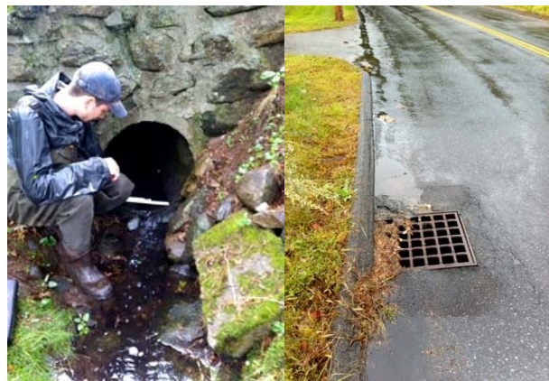
Measuring flow from outfall and stormwater discharging to a catch basin on Wright Road during wet weather sampling.
