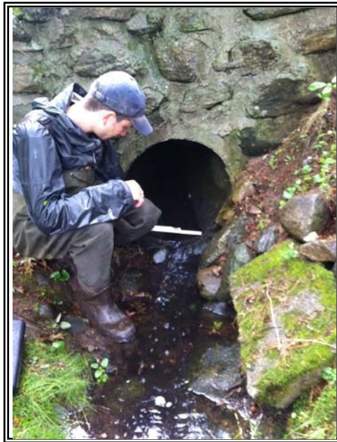
Photograph No. 10: Stormwater sampling at outfall
